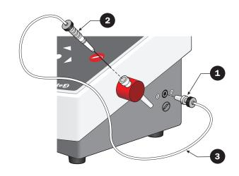
If the unit is reading out of specification, air test showing less than 20.6% O<sub>2</sub> or higher than 21.3% O<sub>2</sub> and you think it requires an air calibration, please contact Technical Support for advice and guidance on how to carry out this procedure.
